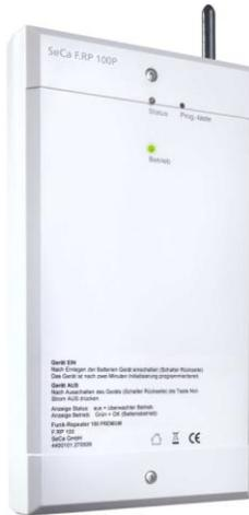
The 100 SHE radio repeaters amplify the radio link between system components and the 3a 100 radio SHE system's control panel, as well as to other repeaters (cascading). It connects to a 230 V power source and includes an emergency power supply. It forwards status alarms and status reports from a maximum of 16 system components and 4 repeaters of the same model. In a SeCa CC100
