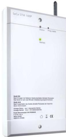
The 100 PREMIUM radio control module can control up to 6 potential-free relay outputs with freely programmable events by means of the CC100 PREMIUM radio fire alarm control panel. It includes a 230V power connection and an emergency power supply. The 100 PREMIUM radio control module is equipped at the factory with 2 relays, and can be expanded to 4 or 6 relays with the plug-in relay
